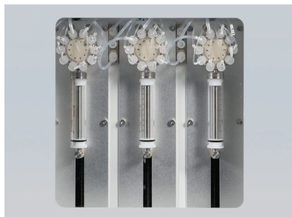
Integrated syringe pump system for a precise and independent control.
