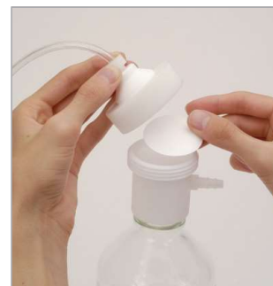
Place membrane filter on top of grid.
