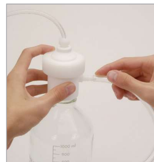
Connect vacuum line to side port.
