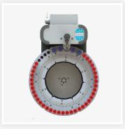
**Load your samples and press START button.** The tray rotates and the arm with needle is aligned on top of the first sample tube to be processed.
